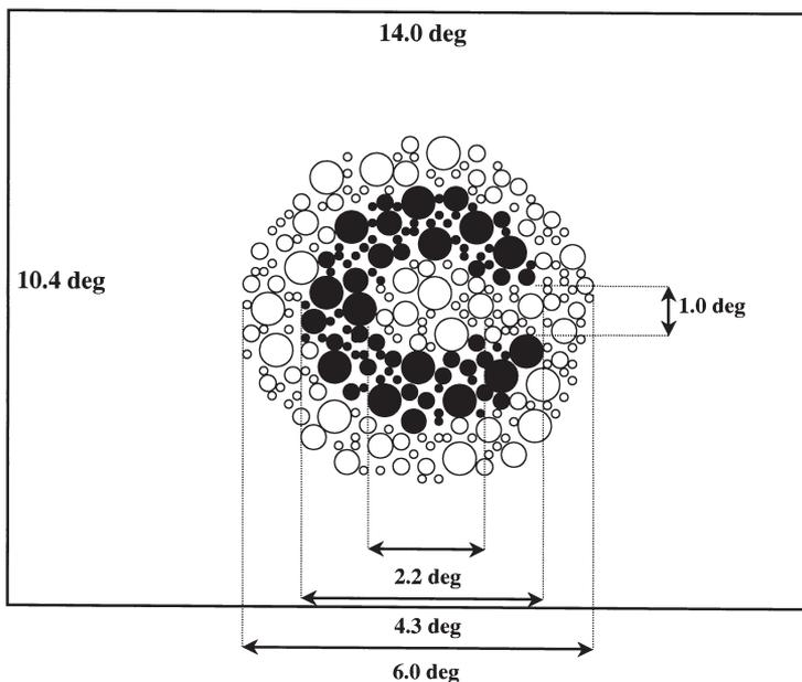
**Figure 1.** Spatial characteristics of C-shaped pseudoisochromatic (PIC) targets developed in this study. Composition is based on the targets of Regan, Reffin and Mollon,<sup>8</sup> with changes in the background chromaticity and starting chromaticities.
