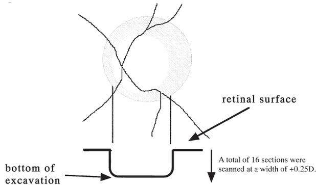
**Figure 1.** Optic scanning method. Total of 16 sections from retinal surface to cup bottom were automatically scanned at width of +0.25 diopter (D). Data on each slice were recorded by videorecorder and digital videotape.
