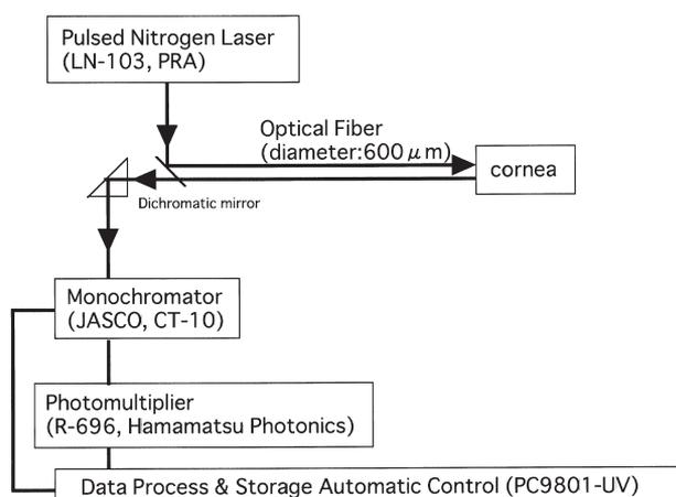
**Figure 2.** Schematic diagram of equipment for nitrogen-pulsed laser spectrofluorometry.
