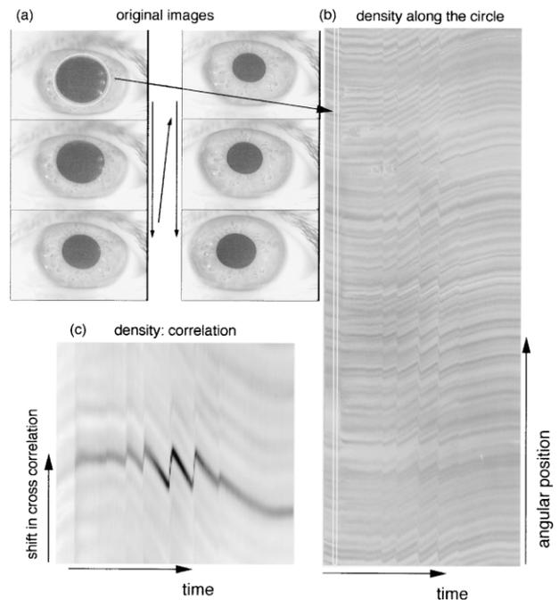
**Figure 4.** Analysis of iris pattern. (a) Original movie. Pupil constriction by light stimulus started at around the third photo. Density distribution along circle just outside pupil (a) is reprojected to one line per image onto another image (b). (b) Torsional eye movement can be read from change in vertical position of horizontal stripes. (c) Cross-correlation function as density with changes in time, and shift between reference and test iris pattern.
