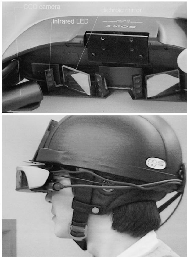
**Figure 1.** Upper: CCD camera set inside head-mounted display (HMD). Lower: HMD with new system worn by a subject. Third camera is not shown.
