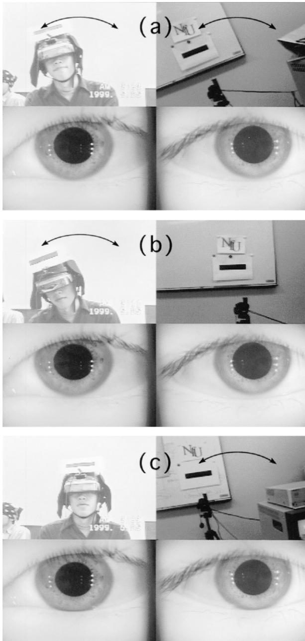
**Figure 3.** Head and image motion in three conditions. (a) See-through compatible mode, (b) head-mounted display (HMD) mode, (c) video mode. Third camera can be seen on HMD in each picture at top left.
