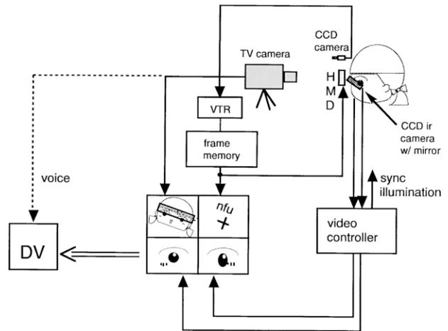
**Figure 2.** Schematic diagram of apparatus. DV: digital video, HMD: head-mounted display, ir: infrared.
