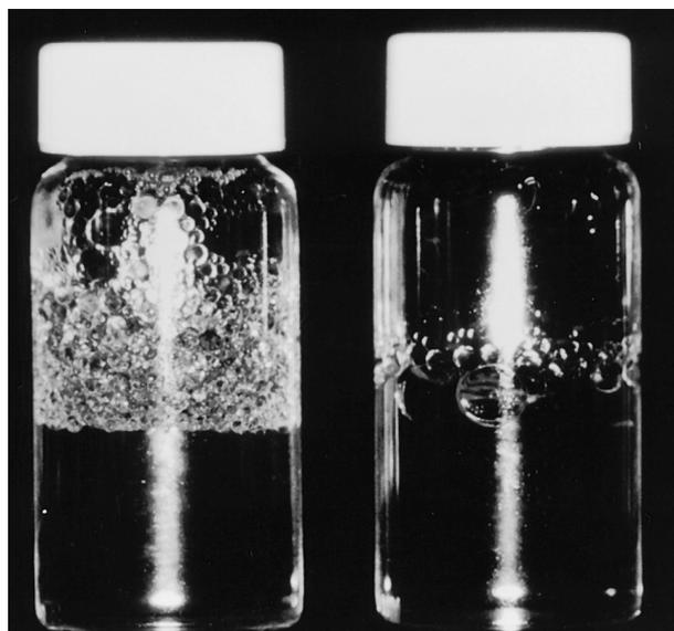
**Figure 3.** When 50-centistoke (cs) silicone oil (SO) or 50-cs silicone-phenylsilicon copolymer (DPC) was shaken horizontally with 1 mg/mL of albumin solution or 1  $\gamma$  globulin solution in completely filled vial, 50-cs SO (left) was almost totally emulsified. However, 50-cs DPC (right) was only slightly emulsified.
