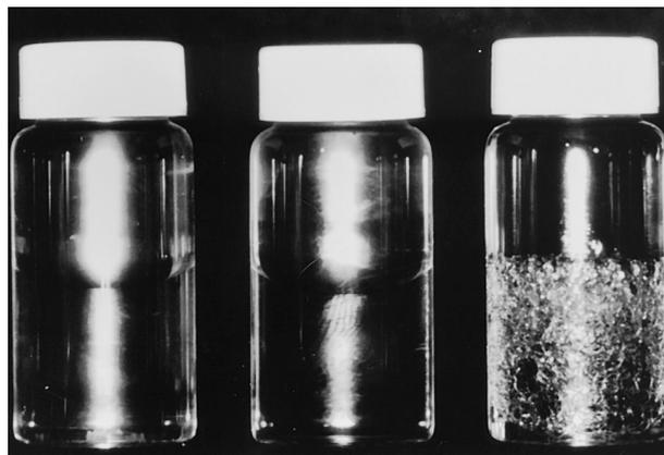
**Figure 2.** When 1,000-centistoke (cs) silicone oil (SO), 1,000-cs silicone-phenylsilicon copolymer (DPC), and 1,000-cs fluorosilicone oil (FSO) were shaken vertically with 1 mg/mL of 1  $\gamma$ -globulin solution in completely filled vial, 1,000-cs SO (left) and 1,000-cs DPC (center) were not emulsified; only 1,000-cs FSO (right) was totally emulsified.
