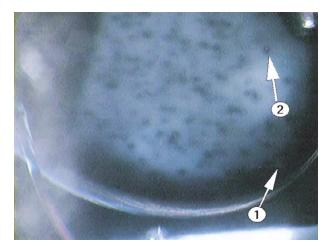
**Figure 6.** Lens after 90 minutes of immersion in 35°C solution. Opacity begins to dissipate from periphery (arrow 1). In center of optic round transparent region containing large glistening particles (arrow 2) remains.
