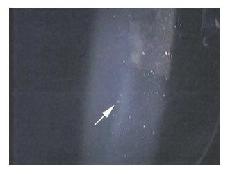
**Figure 9.** Lens after 10 days of immersion in 35°C solution, seen through slit-lamp microscope. Tiny glistenings (arrow) identical to those observed in clinical situations can be seen.
