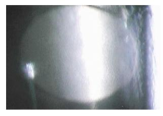
**Figure 4.** Lens in 50°C saline solution. Optic remains clear with no detectable change.
