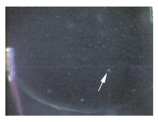
**Figure 7.** Lens after 3 hours of immersion in 35°C solution. Opacity has dissipated but some large glistenings (arrow) remain.
