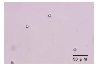
**Figure 10.** Lens after 60 days of immersion in 35°C solution, seen through optical microscope. Microvacuoles measuring 2 to 10  $\mu$ m in diameter are found in optic. They dissipated as lens dried.
